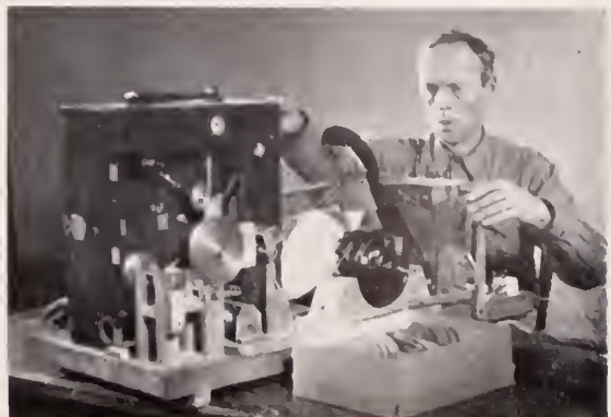
E. Sholpo of Leningrad, sketching the slot-teeth on his discs. These figures are then photographed on the sound path of a moving picture film. It would be truer to speak of "photographic sound" than "designed sound."
